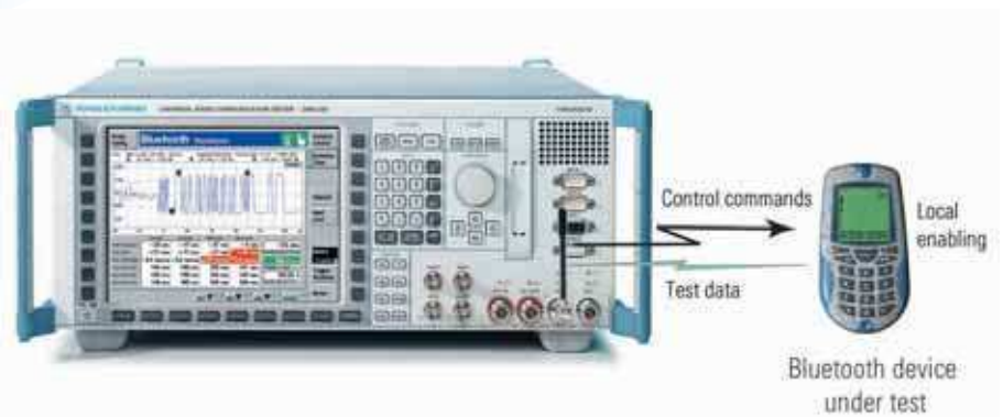
The device under test can be connected to the CMU200 via an RF coupler (antenna) or a cable
